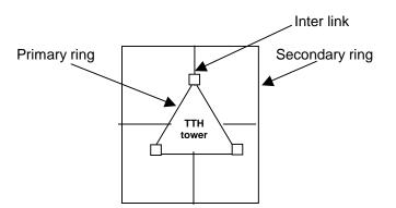
Electrode – GI. Strip 50mm x 5mm x 6 Mtr (standard length) are laid in ring trench and connected to tower leg with lead waster and GI nut bolts bottom of the trench should be filled with sieved good soil up to 10cm height and GI strip should be laid over it.
