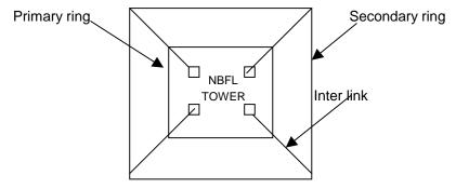
All connections are made by GI nuts and bolts.
